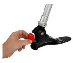
For changing the axial bumpers, first remove one of the axle bolts. Than fully slide out the axle. Plug the axial bumpers into the ankle part.
